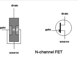
Applying the voltage causes the channel between the source and drain to change size and the amount of current flowing to change
